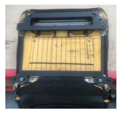
3. Add the front and rear seat brackets. Note there are four square spacers 5mm thick, two for each seat. If you have a VE Commodore seat, place one spacer on each of the front studs. If you have a Falcon seat, place one spacer on each of the back studs before the bracket goes down. The front bracket for both VE and falcon seats look the same and go on the same way (See picture above). Lay the plate down and just put the nuts back on fingertight.
