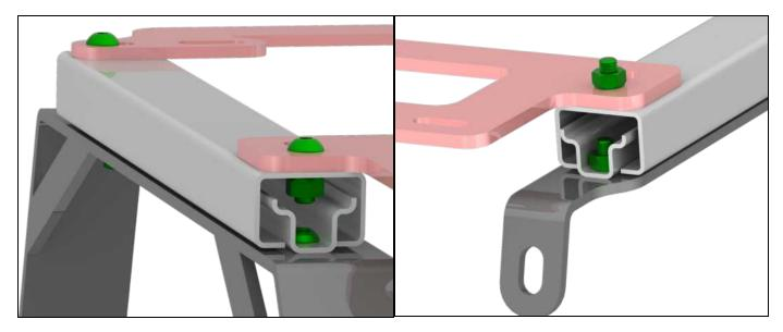
6. Next, centre the two sliding rails to those seat brackets (shown in pink) and set a distance of 440mm between the **middle of each** sliding rail and tighten up the bolts. Recheck that there is a distance of 440mm to the **middle** of each sliding rail after doing up the nuts. You will need to slide the rails back and forth to get access to the nuts and bolts in turn.
